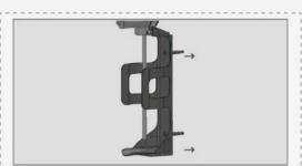
Snap the soap pipe from the dispenser body into the quick connection fitting of the pump.
